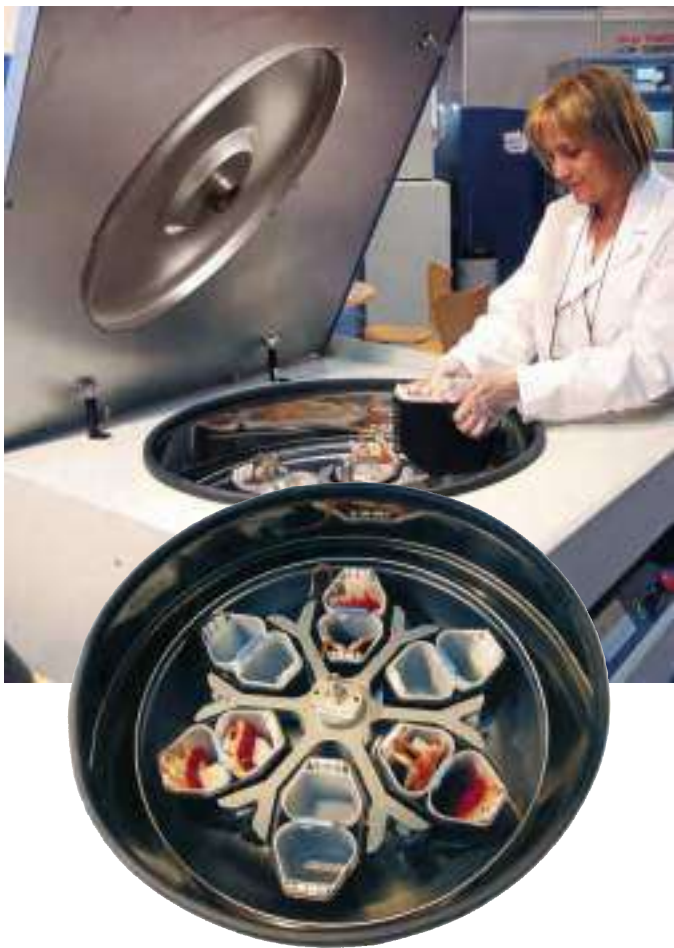
Image showing the rotor and double buckets for quad and triple blood bags of 500 and 800 ml.
