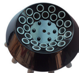
Cabezal angular | GBK022 24×5/10 mL 4000 rpm / 2250 ×g
